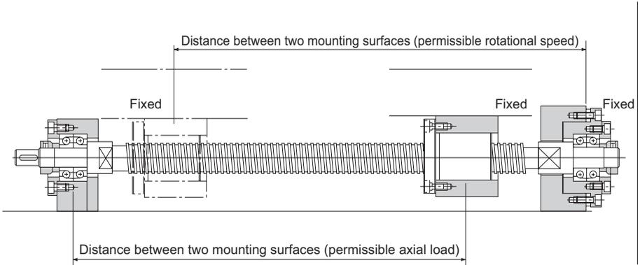
Fig.3 Screw Shaft Mounting Method: Fixed - Fixed
