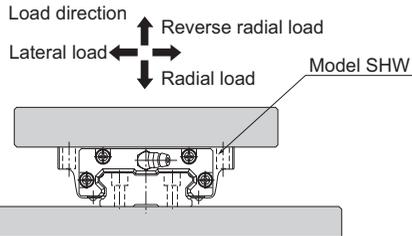
When the minimum possible height of the equipment is allowed (Adjustable preload type)
