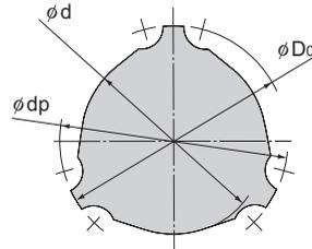
Table1 Sectional Shape of the Spline Shaft
