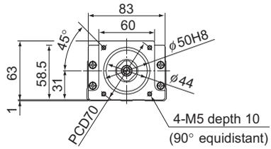
■Housing A for a Separate Motor
