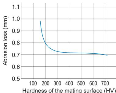
Fig.3 Hardness of the Surface and Wear Resistance
