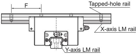
Table2 Dimensions of the LM Rail Tap Unit: mm
