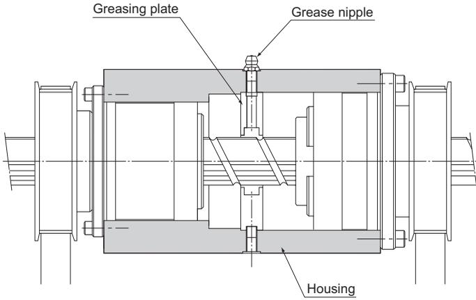
Fig.6 Lubrication Methods
