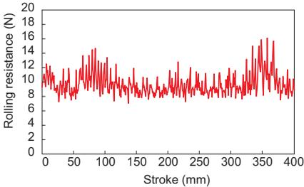
Rolling Resistance Fluctuation Data with HSR25LR
