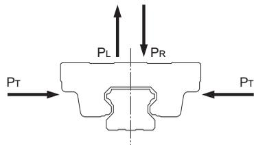
Fig.10 Equivalent of Load of the LM Guide
