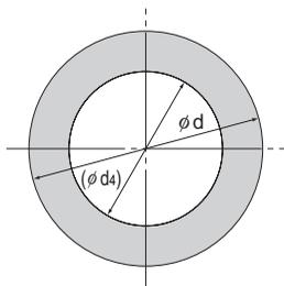
Table1 Dimensions of Hollow LM Shafts
