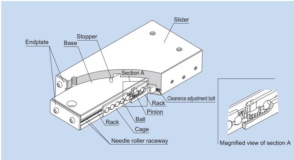
Fig.1 Structure of Linear Ball Slide Model LSP
