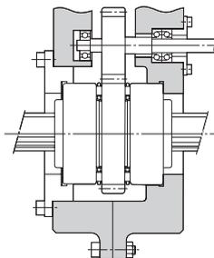
Fig.2 Examples of Fitting the Spline Nut
