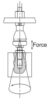
Connecting a rod in the axial direction
