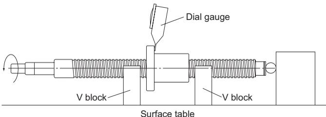
● **Radial Runout of the Nut Circumference in Relation to the Screw Shaft Axis (see Table8 on A-682)**
