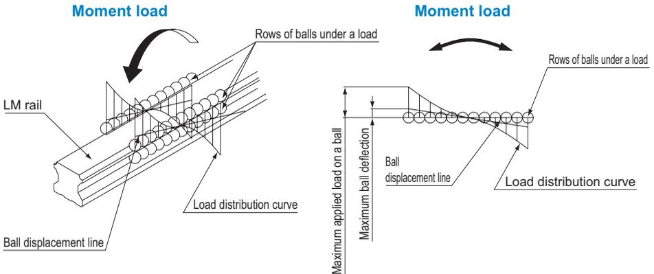
Fig.2 Ball Load when a Moment is Applied
