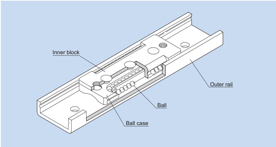
Fig.1 Structure of Precision Linear Pack Model ER
