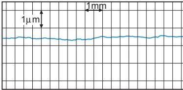
After travel (no fretting corrosion observed)
