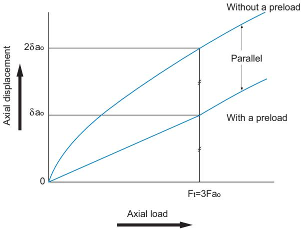
Fig.4 Elastic Displacement Curve of the Ball Screw
