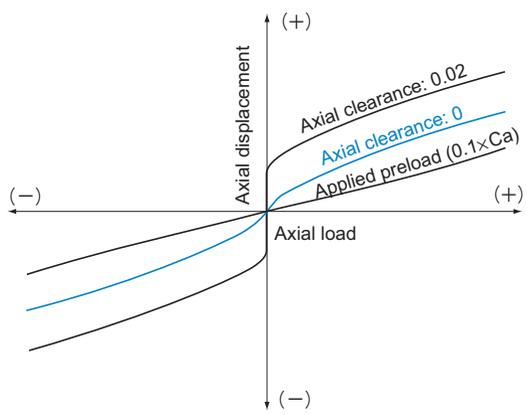
Fig.6 Axial Displacement in Relation to Axial Load
