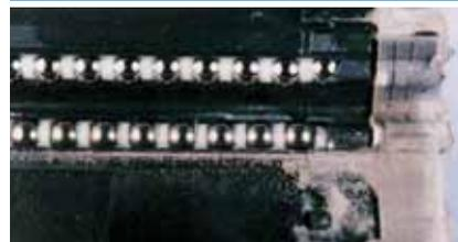
No foreign matter entering the raceway observed
