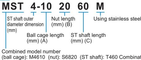
Note) The model numbers of ball cage, nut and ST shaft are indicated in the corresponding specification table.
