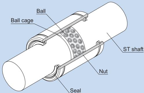
Fig.1 Structure of LM Stroke Model ST
