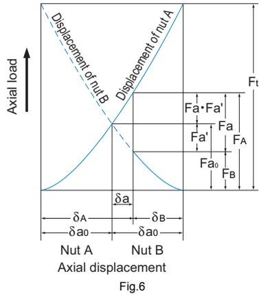
Nuts A and B are provided with preload  $F_{a_0}$  from the spacer. Because of the preload, nuts A and B are elastically displaced by  $\delta_{a_0}$  each. If an axial load ( $F_a$ ) is applied from outside in this state, the displacement of nuts A and B is calculated as follows.
