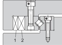
When high accuracy and high rigidity are required, use tapered gibs 1 and 2.
