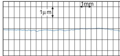
After travel (fretting corrosion observed)
