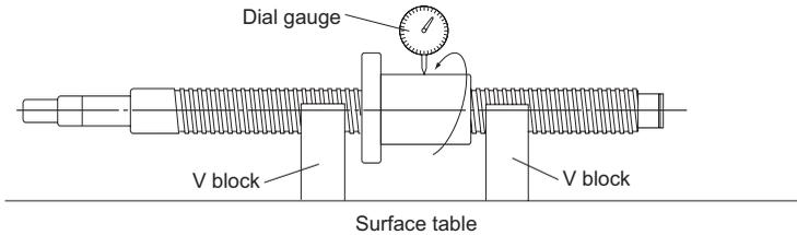
● **Parallelism of the Nut Circumference (Flat Mounting Surface) to the Screw Shaft Axis (see Table9 on A-682)**
