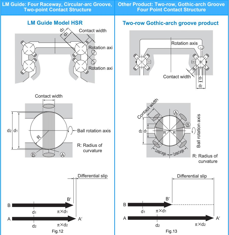
As indicated in Fig.12 and Fig.13, when the ball rotates one revolution, the ball slips by the difference between the circumference of the diameter of inner surface ( $\pi d_1$ ) and that of the outer contact diameter ( $\pi d_2$ ). (This slip is called differential slip.) If the difference is large, the ball rotates while slipping, the friction coefficient increases more than 10 times and the friction resistance steeply increases.
