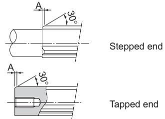
Fig.1 Chamfer A
