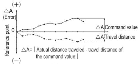
Fig.10 Positioning Accuracy
