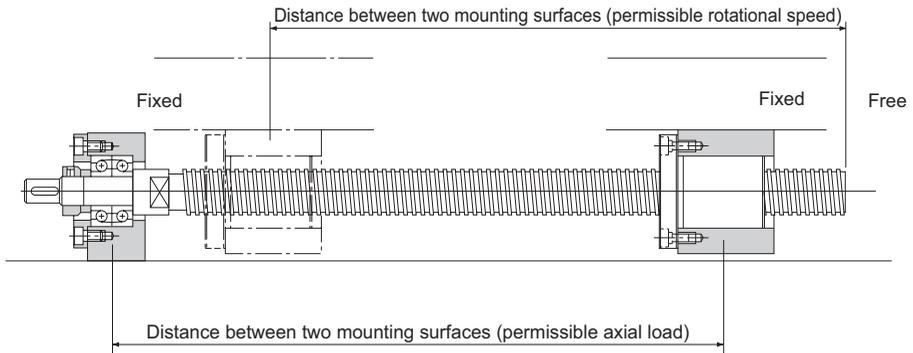
Fig.1 Screw Shaft Mounting Method: Fixed - Free
