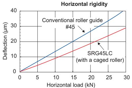
Rigidity is measured with the two axes placed in parallel and one of the axes not fixed with a bolt in order not to apply a moment.
