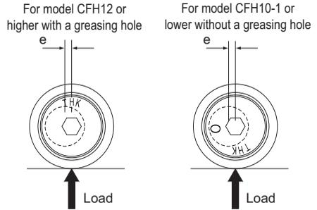
The figure shows the position of the THK logo in relation to the eccentricity direction for model CFH12 or higher with a greasing hole.
