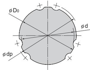
Table1 Sectional Shape of the Spline Shaft
