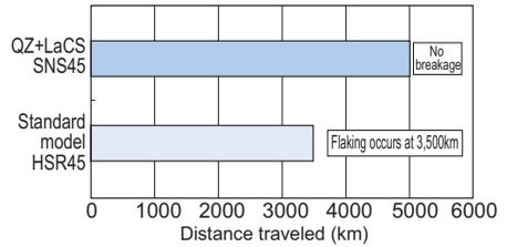
\* When using the LM system under severe environment, use QZ Lubricator and Laminated Contact Scraper LaCS (see "Laminated Contact Scraper LaCS" on A-353) in combination.
