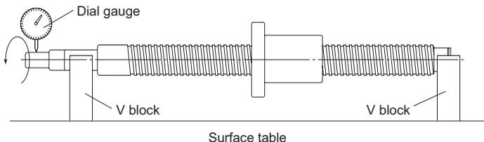
● **Radial Runout of the Circumference of the Thread Root in Relation to the Supporting Portion Axis of the Screw Shaft (see Table5 on A-681)**
