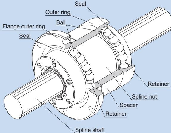
Fig.1 Structure of Rotary Ball Spline Model LTR
