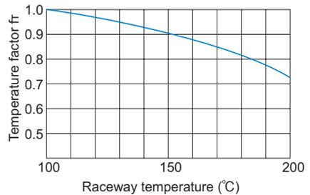
Fig.2 Temperature Factor (f<sub>T</sub>)
