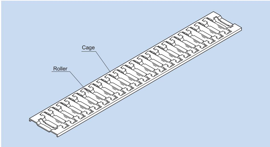
Fig.1 Structure of LM Flat Roller Model FT
