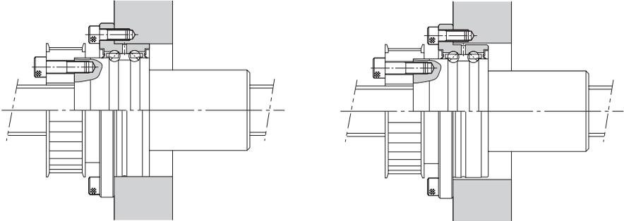
Installation to the housing can be performed on the end face of the outer ring flange.
