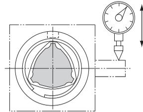
Fig.7 Measurement of Clearance in the Rotational Direction
