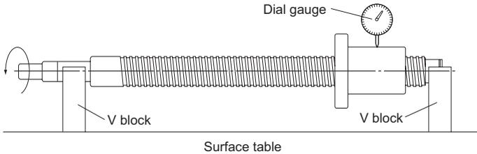
● **Perpendicularity of the Supporting Portion End of the Screw Shaft to the Supporting Portion Axis (see Table6 on A-682)**
