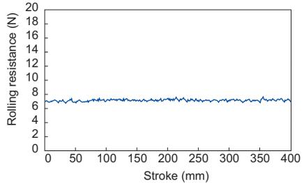
Rolling Resistance Fluctuation Data with SHS25LV
