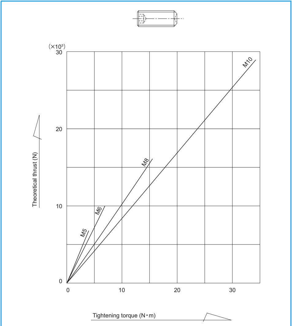
Note) The theoretical thrust may vary depending on the lubrication and the conditions of the surfaces of the setscrew or the reference surface ( $\mu = 0.13$ ).
