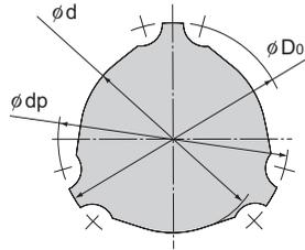
Table1 Sectional Shape of the Spline Shaft
