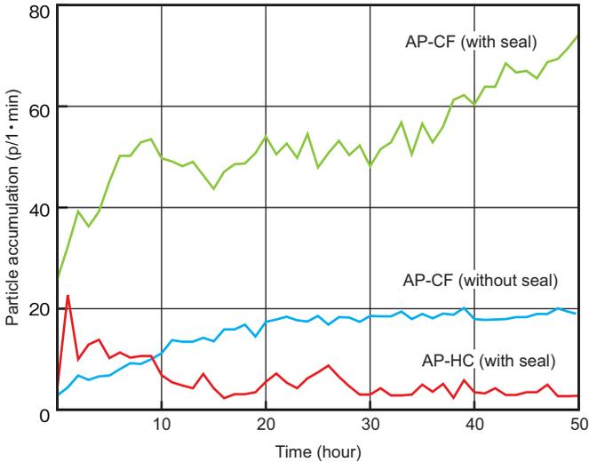
THK AP-HC treatment provides high surface hardness and has high wear resistance. The high level of wear in the early stage in the graph above is considered to be due to the initial wear of the end seal.
