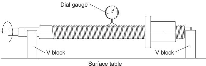
Note) For the overall radial runout of the screw shaft axis, refer to JIS B 1192-1997.
