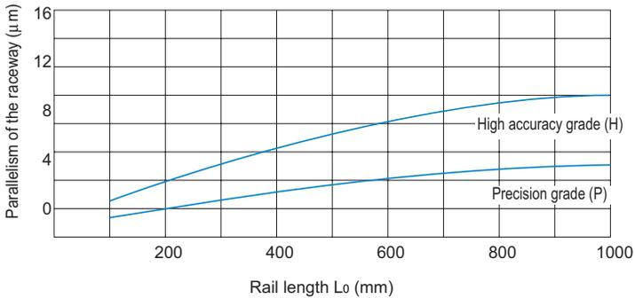
Fig.4 Rail Length and Parallelism of the Raceway
