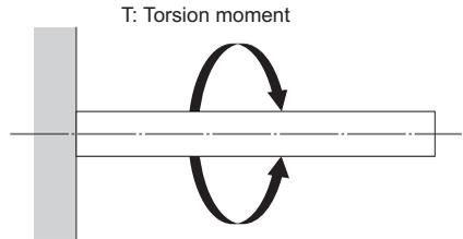
**[When the Spline Shaft Simultaneously Receives a Bending Load and a Torsion Load]**
