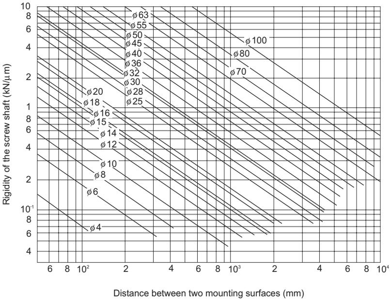
Fig.11 Axial Rigidity of the Screw Shaft (Fixed-Fixed)
