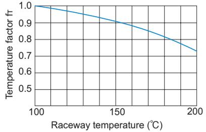
Fig.2 Temperature Factor (f<sub>t</sub>)
