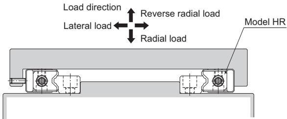
When a medium load is applied and the mounting surface is rough (Preload, self-adjusting type)
