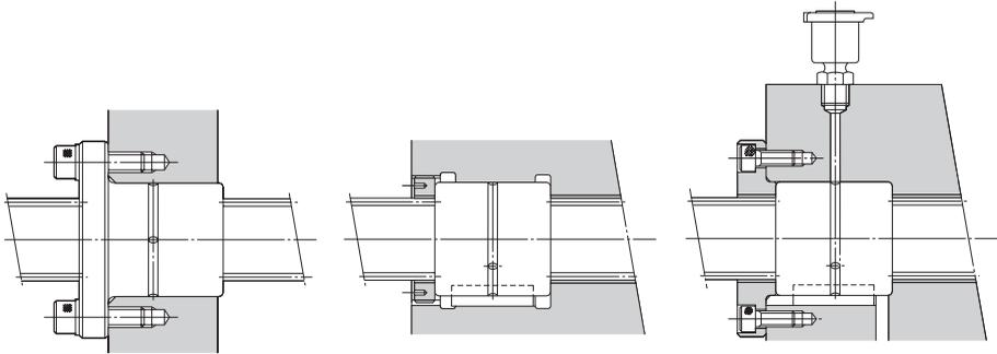
Fig.3 Examples of Installing the Lead Screw Nut
