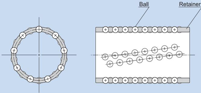
Fig.1 Structure of Die-setting Ball Cage Model KS
