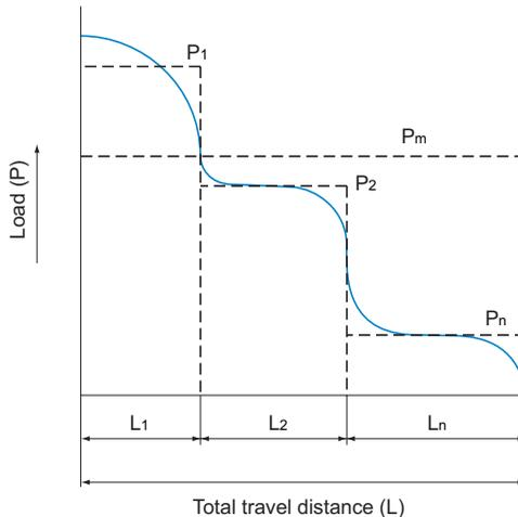
(2) When the load fluctuates monotonically
