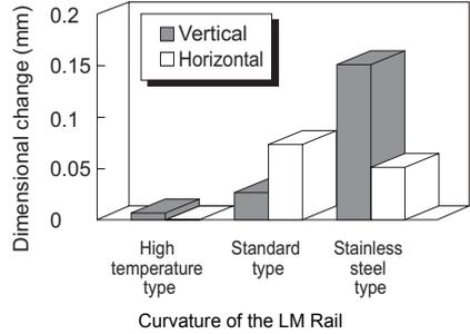
Note1) The above data on overall length and curvature indicate dimensional change when the LM rail is cooled to normal temperature after being heated at 150°C for 100 hours.
