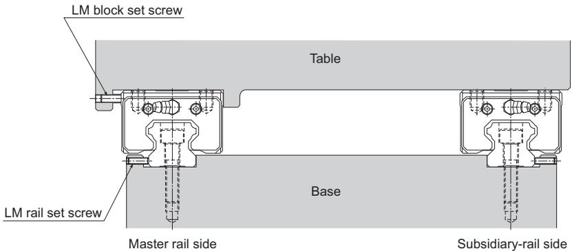
Fig.1 When the Machine Receives Vibrations or Impact
