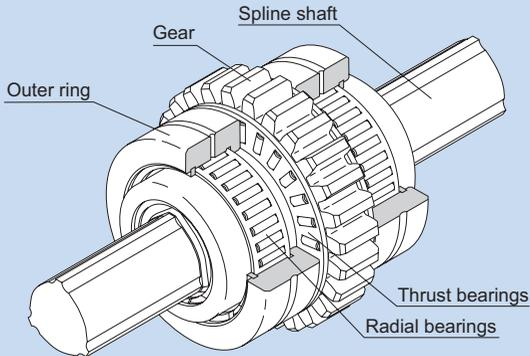
Fig.1 Structure of Rotary Ball Spline Model LBG
