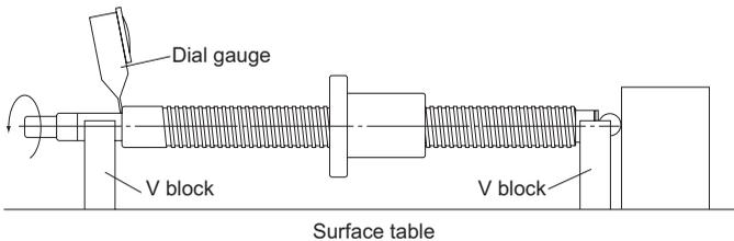
● **Perpendicularity of the Flange Mounting Surface of the Screw Shaft to the Screw Shaft Axis (see Table7 on A-682)**
