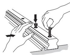
Fig.4 Checking with the Bolt for an Allowance
