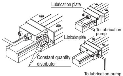
Fig.1 Structural Drawing
