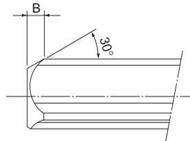
Fig.2 Chamfer B
