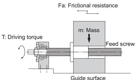
● Thrust Generated When Torque is Applied
