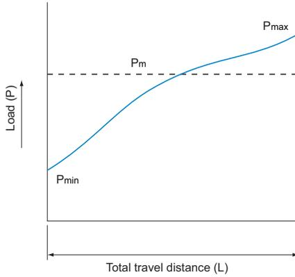
(3) When the load fluctuates sinusoidally
