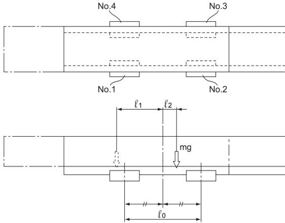
**[Load Applied to the LM Block]**
