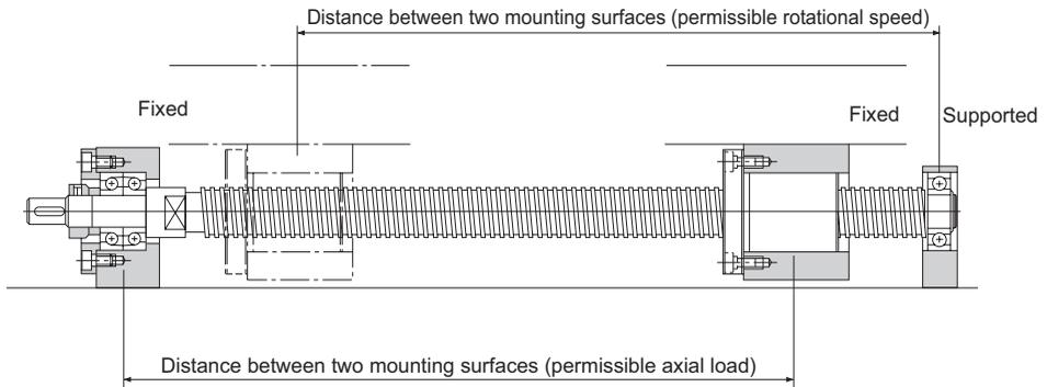
Fig.2 Screw Shaft Mounting Method: Fixed - Supported
