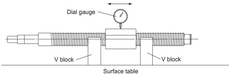
● **Overall Radial Runout of the Screw Shaft Axis**
