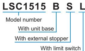
Note) Unit base, external stopper and limit switch are not available for model LSC1015.
