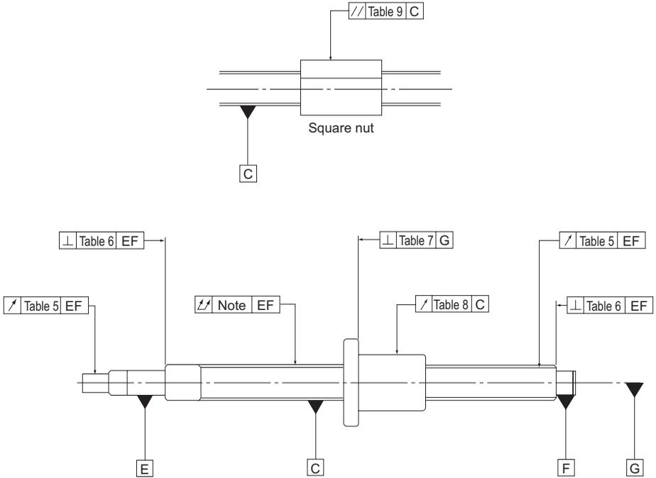
Note) For the overall radial runout of the screw shaft axis, refer to JIS B 1192-1997.
