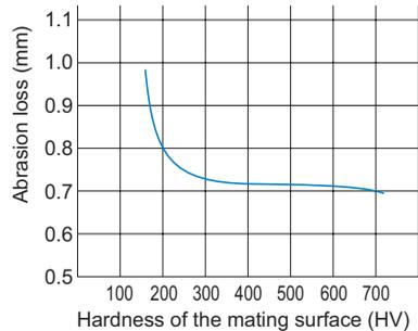
Fig.3 Hardness of the Surface and Wear Resistance
