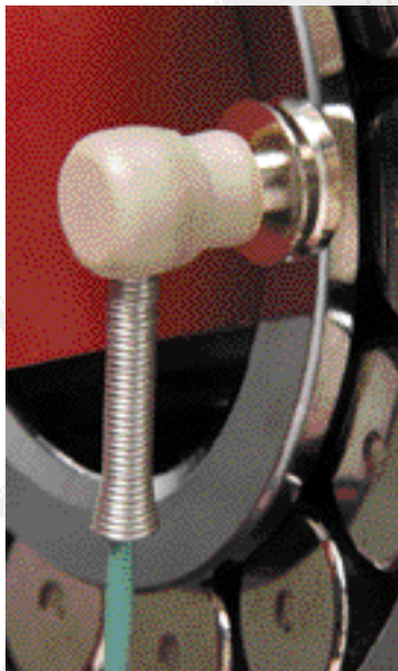
Magnetic temperature probe. (a clamp probe is also available for non-ferrous components).
