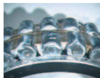
Photo. 6.2 Filling grease into cylindrical roller bearing
