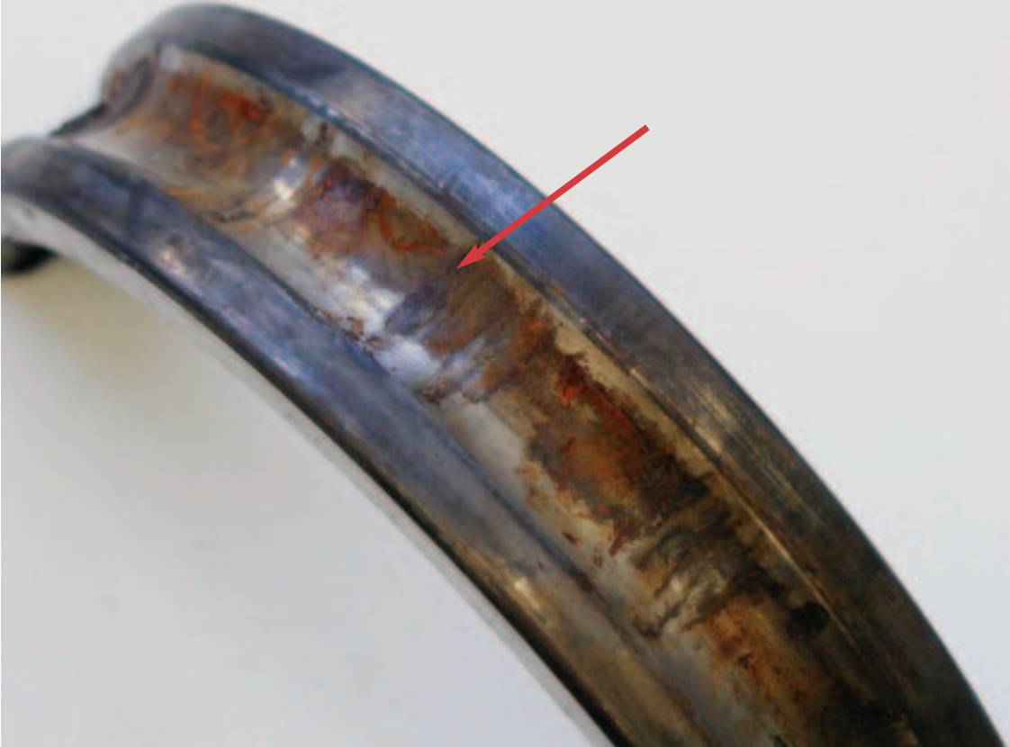
Wear due to external vibration when the bearing is not operating – False Brinelling
