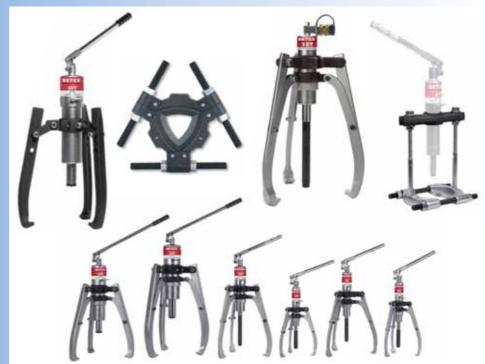
Hydraulic pullers 25-100 t cap., self-centering, mobile
