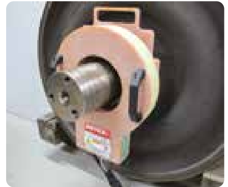
Heating labyrinth rings for dismounting
