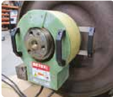
Heating bearing rings for dismounting
