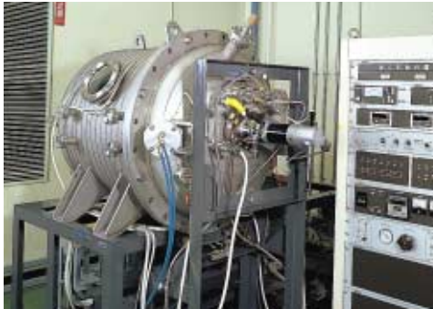
Photo 1-4-1 Vacuum testing system
