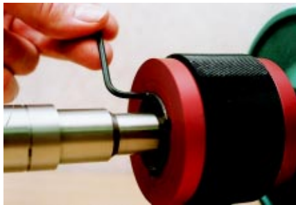
Tighten screws alternately.
