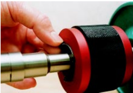
Tighten screws finger tight.
